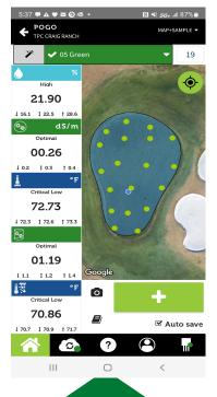
Each new moisture, salinity (EC), temperature and salinity index measurement is colorcoded to clearly display where your conditions are in relation to your customized target range.
